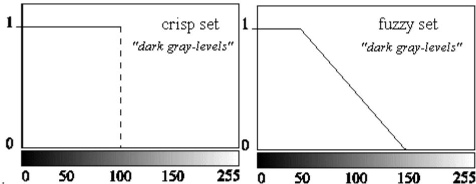
**Gambar 2.1** Representation of "dark gray-levels" with a crisp and a fuzzy set (Adapted from: Tizhoosh, Fuzzy Image Processing, ©CopyRight Springer,1997)
